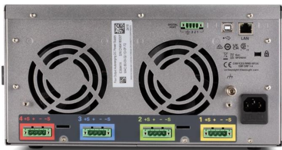
Figure 12. LAN and USB are standard connectivity on E36441A
