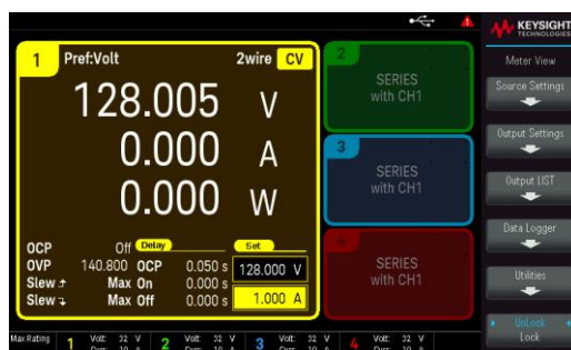
Figure 3: Increase output voltage with E364SNP kit.
